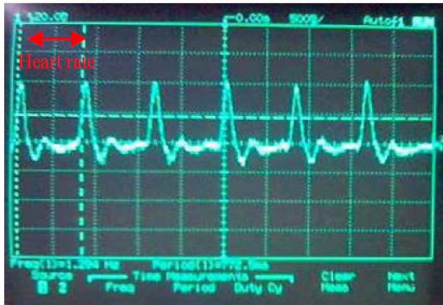
Figure 2 Pulse rate results captured on an oscilloscope using the MMSB method [1].
